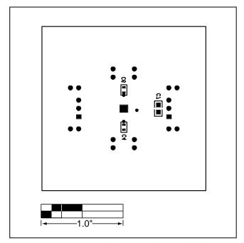
Figure 5. MAX9710 EV Kit Component Placement Guide— Solder Side
