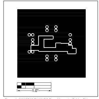
Figure 6. MAX9710 EV Kit PC Board Layout—Solder Side
