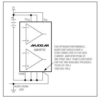
Figure 1. MAX9710 Audio Ground Connection
