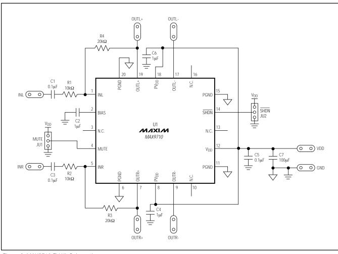
Figure 2. MAX9710 EV Kit Schematic
