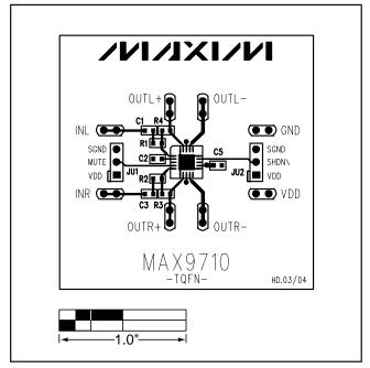
Figure 3. MAX9710 EV Kit Component Placement Guide—Component Side
